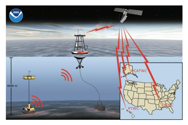
Figure 5. Deep Ocean Assessment and Reporting of Tsunami (DART) tsunameter technology.
